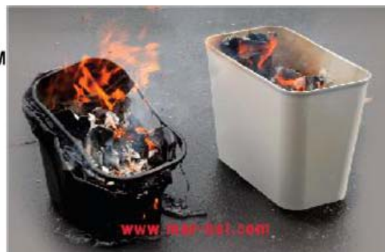
Testing result of plastic (left) and Waste-Safe™ (right) Estimated elapsed time: 1 min, 30 sec
